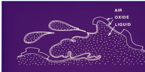
surface flooding and formation of bi-film
